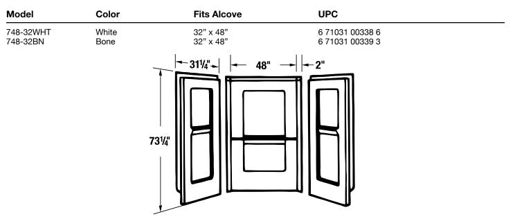
**General:** Furnish and install as shown on plans, 32" x 48" rectangular shower, DURAWALL<sup>®</sup> Shower Walls Model 748-32, as manufactured by E.L. Mustee & Sons, Inc. Shall be 3-piece, molded fiberglass wall with minimum thickness of 125 mils and mounts direct-to-studwalls. Includes center panel with molded-in shelves and two side panels with molded-in shelf. Self aligning panels use a tongue-and-groove connection. Shall meet ANSI Z 124-2011.2. Color\_\_\_\_(White, Bone).
